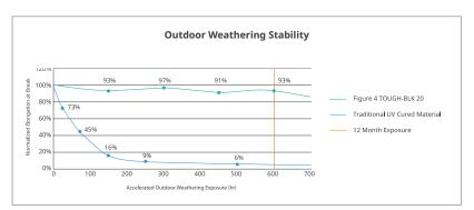
Performed in accordance with ASTM G154 to simulate actual outdoor exposure of plastics
