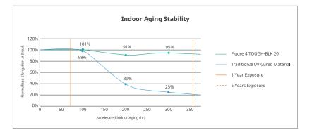
Performed in accordance with ASTM D4329 to simulate ASTM D4459, Indoor exposure of plastics from solar radiation through a window
