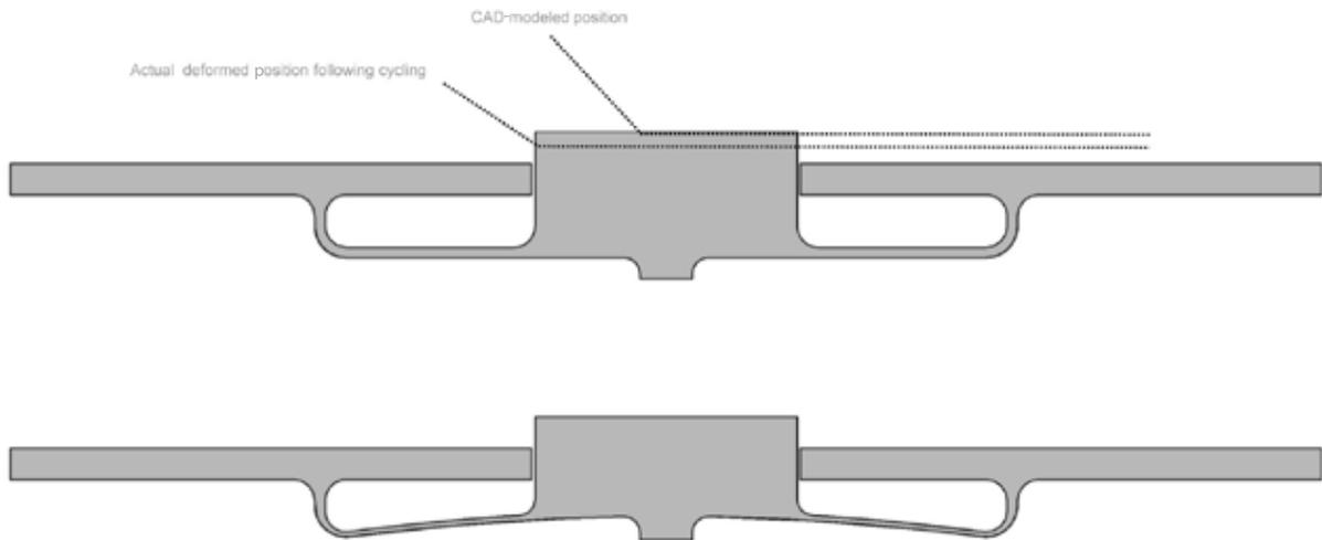
There are many different approaches to integrated button design. Allow at least 0.3mm clearance between the button and the slot or hole from which it emerges to prevent fusing. You should also CAD model the button to be higher than the final desired position, as the nylon “leaf springs” will tend to deform into a slightly depressed position. For example, if you want the button to be flush with the surface and CAD model it as such, you will find that it will
