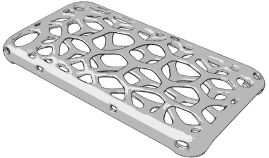
Also note that while you may cut down on the weight of the final part relative to a solid non-grid section, you will increase cleaning time and you will increase draw time on the systems, as the laser now outlines and fills in the feature rich cross-sections.
