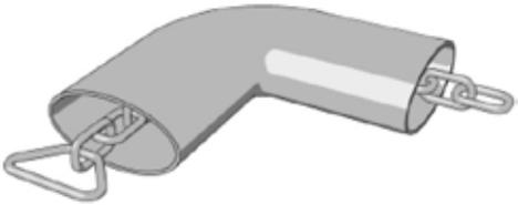
Consider CAD modeling in a chain through the duct. When finishing, a quick pull of this chain through the duct will clear an open channel for the bead blasting media to get a good cleaning velocity in the duct.
