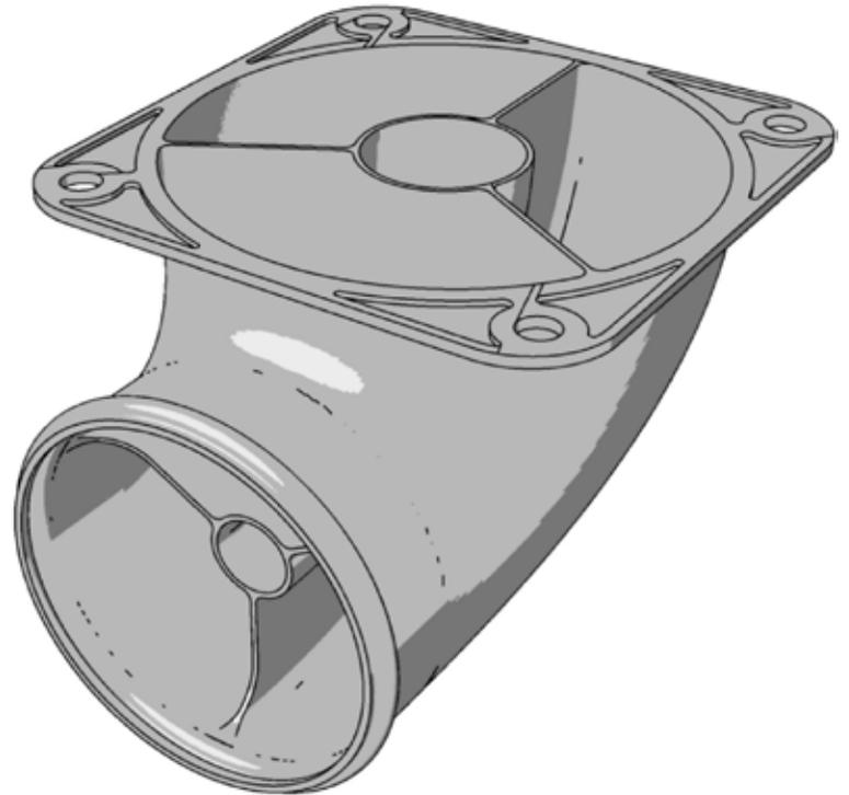
Always apply generous fillets to baffles to prevent side walls of ducts from splitting, especially if component will be exposed to pressure and/or cycling of temperature.
