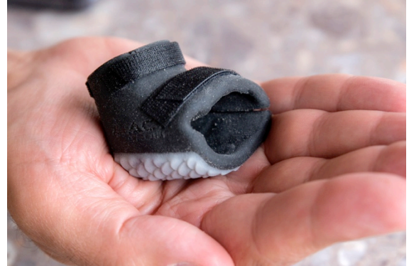
The lightweight and flexible orthotic boot was printed in the ProJet® MJP 5500X multi-material 3D printer as a single piece
