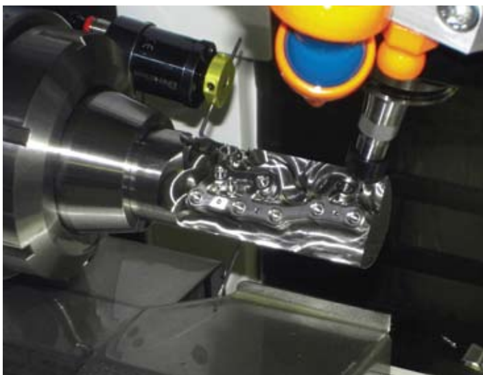
Willem-Macodel 408MT doing a five-axis swarf cut to finish the perimeter of a titanium orthopedic plate at TraTek.
