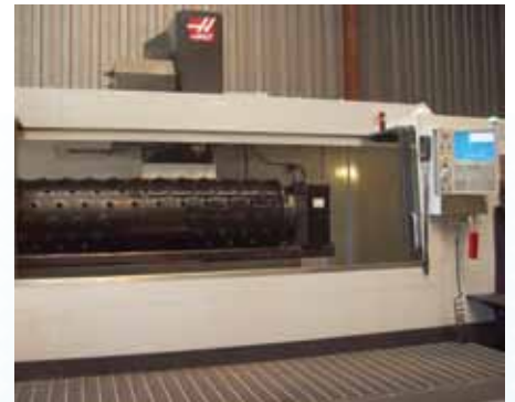
Machining the header requires boring numerous holes of small diameters at specific angles and precise locations. Repeatability and 0.100" true position tolerance from three datum required machining the holes in a single set up, which Taylor Forge does on this Haas VF11 4-axis vertical mill.
