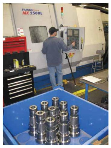
This turning center features live tooling capability. Another turning center for still smaller bits features live tooling and a secondary spindle.
